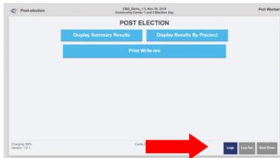
Tap the **Shut Down** button in the lower right corner of the screen. The ClearCast machine will turn off automatically. Tap **Submit** to confirm.
