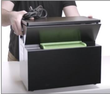
2. Lift the lid/screen on the top of the scanner.
